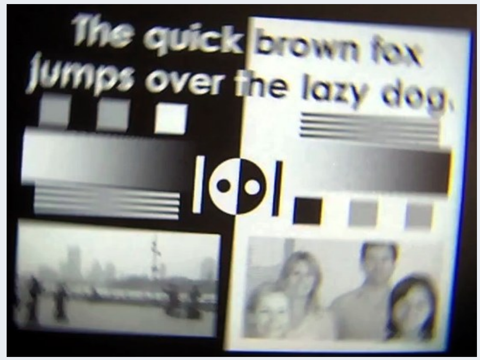
(b) 22,727 Hz binary projector (using our binary image generation algorithm)
