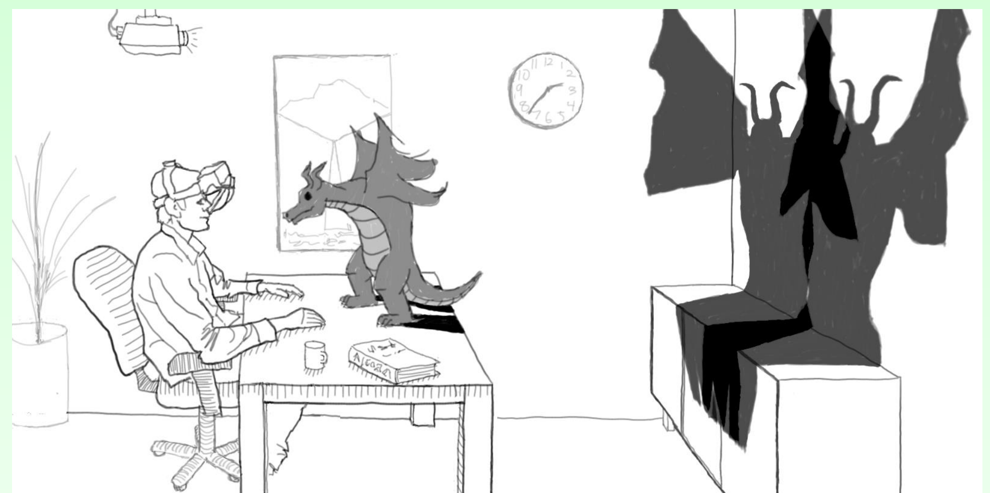
Figure 5: Concept drawing illustrating a virtual dragon appearing solid on the user's desk. Projector lighting creates the occluded view. The dual shadows are presented to each eye separately.
